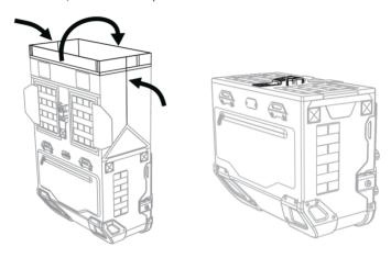
5. Fasten to the motorcycle side rack, buckle the side fixed lock buckle.
