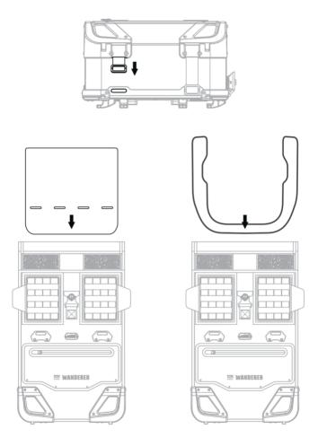
4. Fold the sides of the bag inward, bend the bag once and glue the Velcro downwards, and fasten the top buckle.
