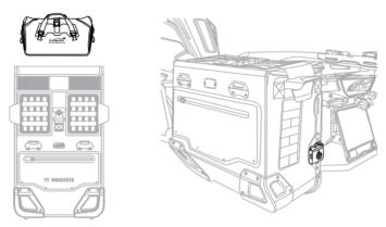
2. Fix the waterproof bag on the motorcycle waterproof side bag with a quick-release strap.
